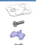
Place the 8-32 countersunk bolts in their proper positions on  $a1\_o.stl$ . Three of them will be locked in place beneath the palm pad upon assembly of the palm pad to  $a1\_o.stl$ .
