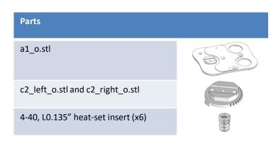
Install the remaining heat-set inserts in the finger base parts:  $a1\_o.stl$ ,  $c2\_left\_o.stl$ ,  $c2\_right\_o.stl$ . Note that  $c2\_left\_o.stl$  and  $c2\_right\_o.stl$  are mirrors of each other, so they are not interchangeable.
