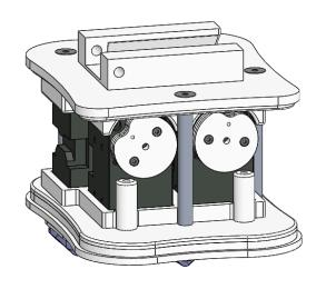
For each finger sub-assembly with base, regardless if it is Pivot-Flexure or Pivot-Pivot, it is attached to the hand frame with two 4-40 countersunk bolts.
